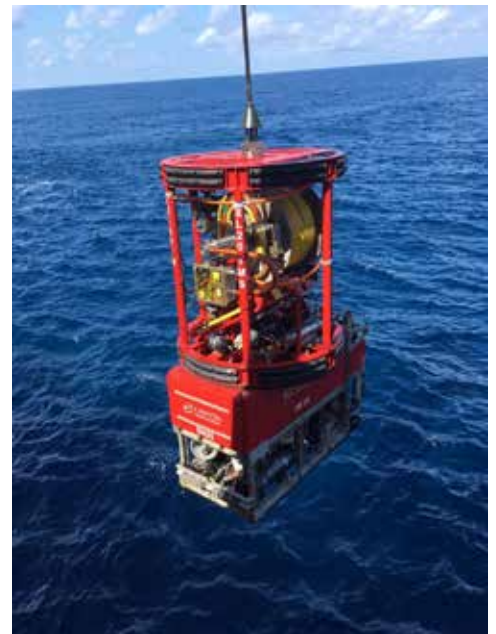
Scorpion SN20, a Work-class Remotely Operated Vehicle (WROV) performing subsea inspection activities
