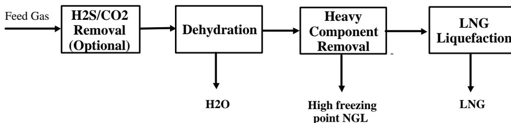
Figure 3 - Block diagram for typical LNG plant
