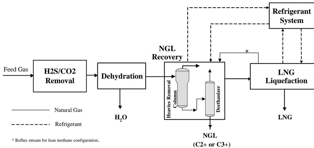
Figure 4 - Block diagram showing the integrated NGL and LNG process
