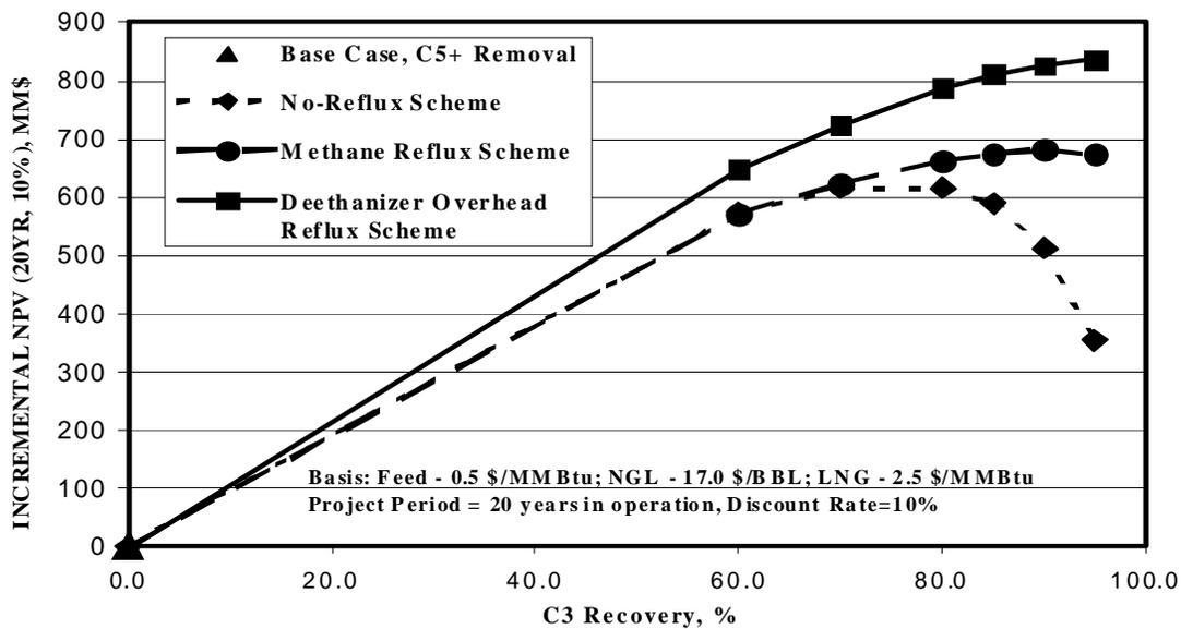
Figure 6 - Incremental NPV at Varying Propane Recovery for Differing Integrated Cases
