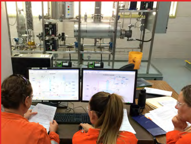
Trainees operating a gas absorption rig
