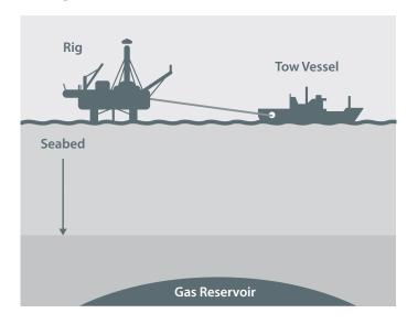
A drilling rig is towed to the drilling location.
