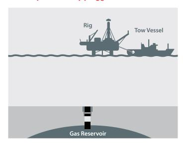
Cement plugs are placed within the well as part of a process called plug and abandonment. The marine riser, BOP and wellhead are removed so no equipment is protruding from the seabed. The anchors are then removed so the drilling rig can be towed to the next drilling location or demobilised from the area on completion of the program.
