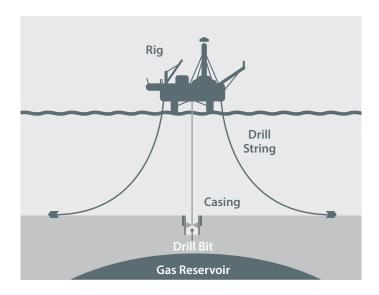
The top hole is drilled and then cased with cement and steel. The top hole is approximately 1m in diameter.
