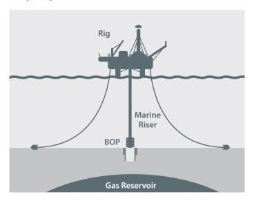
The marine riser returns drilling fluids and cuttings to the drilling rig for reconditioning, recirculation and/or discharge. The BOP is an assembly of specialised safety valves put in place before drilling into the reservoir and is used in the unlikely event of an emergency to control well pressure and prevent a loss of well control release.
