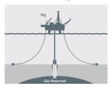
In the event that a gas reservoir is discovered, the well may be tested by flowing gas to the surface for analysis and then flaring through the flare boom.
