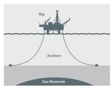
Anchors are laid on the seabed and can be laid prior to or on arrival of the drilling rig.
