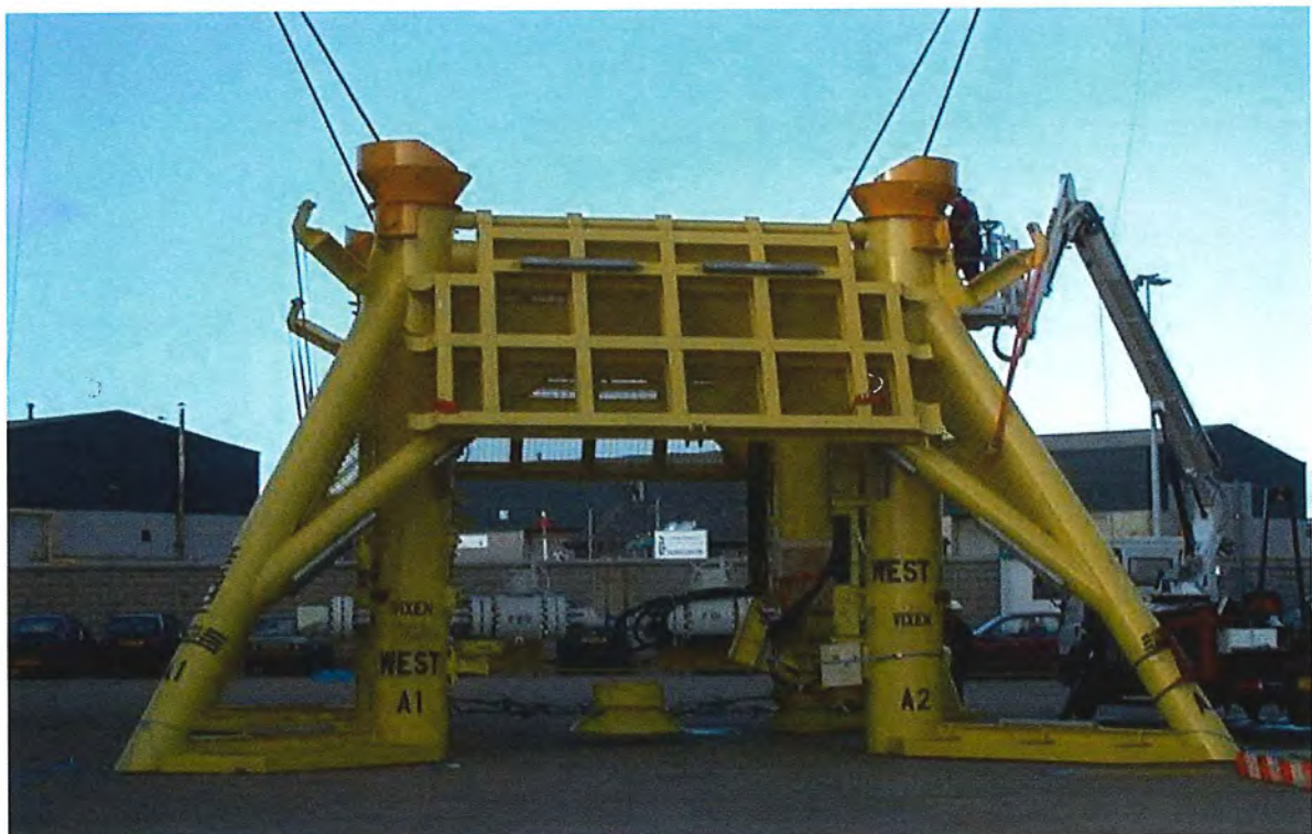
Figure 2.2.1 Photograph of subsea manifold, Vixen VM
